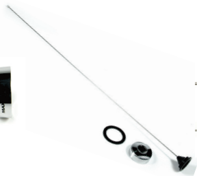
PCTCN1520 (MHB1520) Antena 1/4, ganancia unitaria, 150-162 MHz
