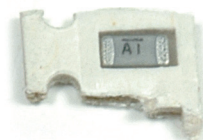
2111078B25 Capacitor RF 27 5 NPO 100V
